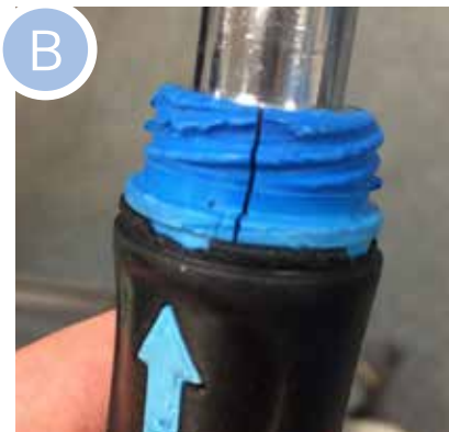
Camera - electrical connector is physically damaged
