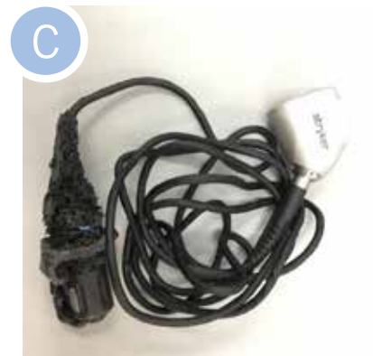
Camera - cable is kinked and melted
